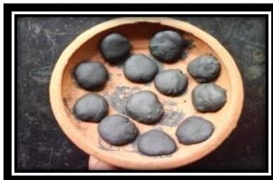
**3 Before Igniting Process – Pellets of Mica**
